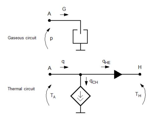
The diagram shows that the heat flow q to the chamber consists of two components:
