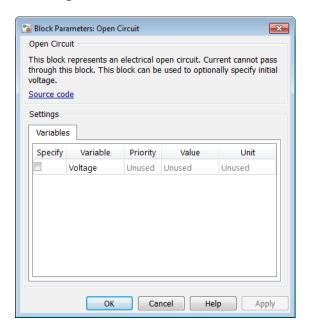
The Open Circuit block has no parameters.
