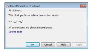
The PS Subtract block has no parameters.
