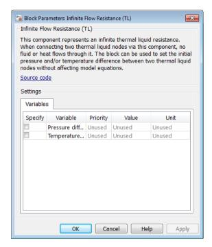
The Infinite Flow Resistance (TL) block has no parameters.
