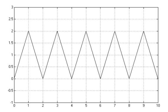
Discrete — Each linear segment in the repeating sequence is defined by its duration and start value. The end value of a segment is the same as its start value.
