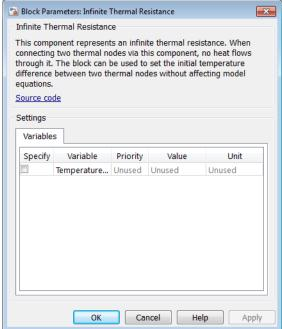
The Infinite Thermal Resistance block has no parameters.
