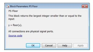
The PS Floor block has no parameters.
