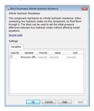
The Infinite Hydraulic Resistance block has no parameters.
