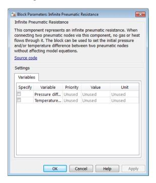
The Infinite Pneumatic Resistance block has no parameters.
