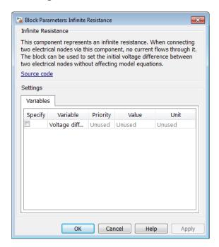
The Infinite Resistance block has no parameters.
